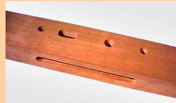
Machinings for a lock casing
