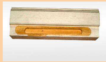
Routing for striker plates
