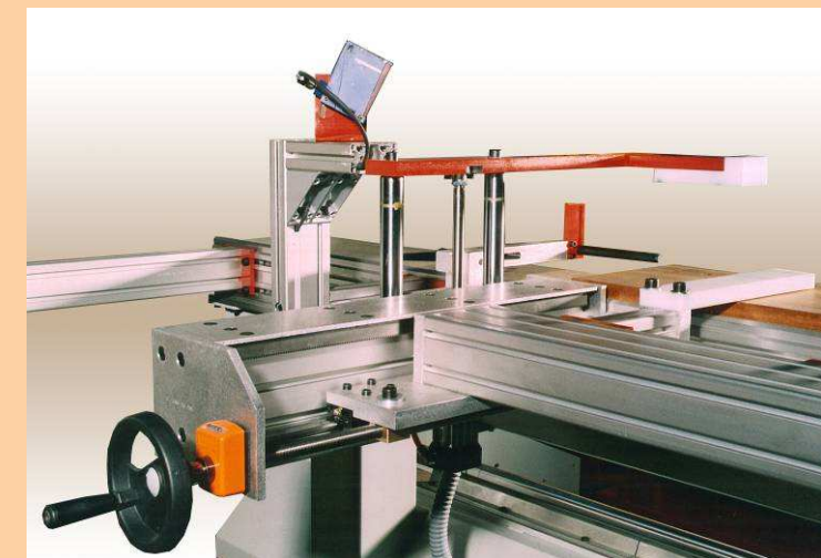
Detailed view of the table equipped with a backing ruler that allows to position the parts in counter-reference. It avoids the stops on the machining side, thus avoiding collisions.
