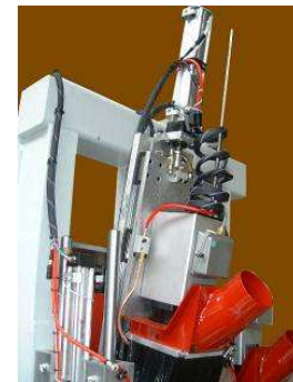
Tilted drilling unit for drain making
