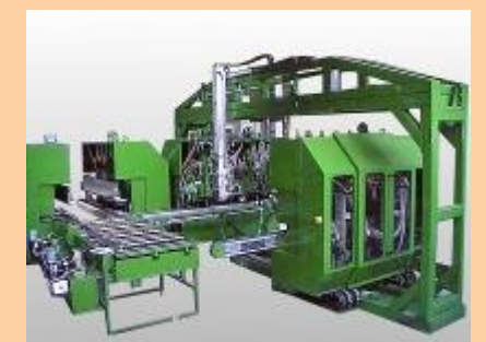
Calibrating line for polyurethane panels
