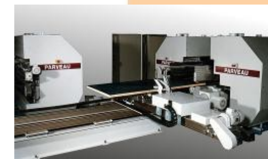
Calibrating line for flush doors
