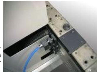
View of the reference detector and a conveyor chain with a Standard stopper
