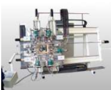
CNC drilling, screwing, and framing machine for windows with mechanical assembling
