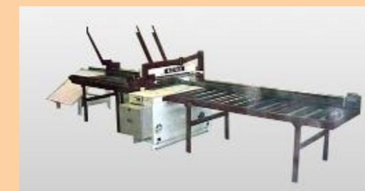
TEP equipped with a free roller entry table, a free roller exit table, a ruler with 3 pneumatic retractable stops, and a tilted evacuation table.
